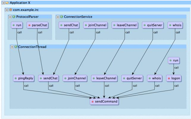
Figure 11: Call graph of `sendCommand()`. Only the first two levels from the original graph are shown here.
