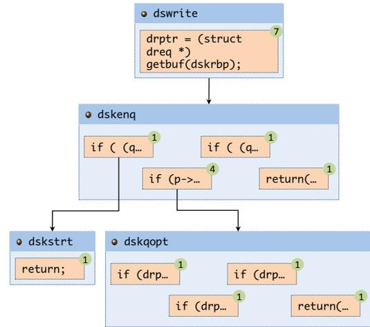
Figure 5: Call graph of `dswrite()` restricted to the memory leak analysis.
